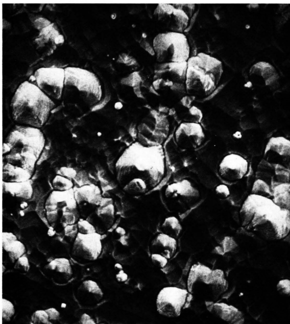
Fig. 1. Scanning electron micrograph of tilted surface of copper alloy containing 85 wt.% copper and 5 wt.% each of zinc, tin and lead.
